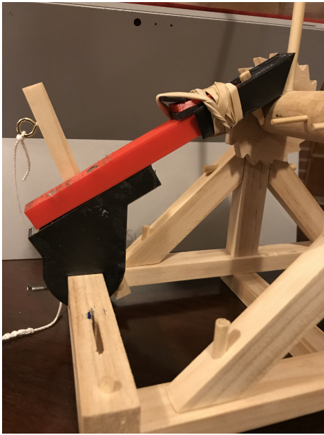
Figure 2: 3D printed bumper
