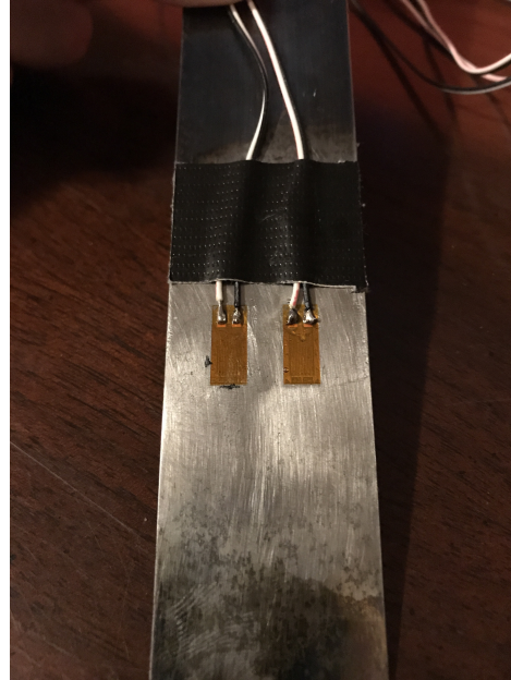
Figure 3: Installed strain gauges with relief tape
