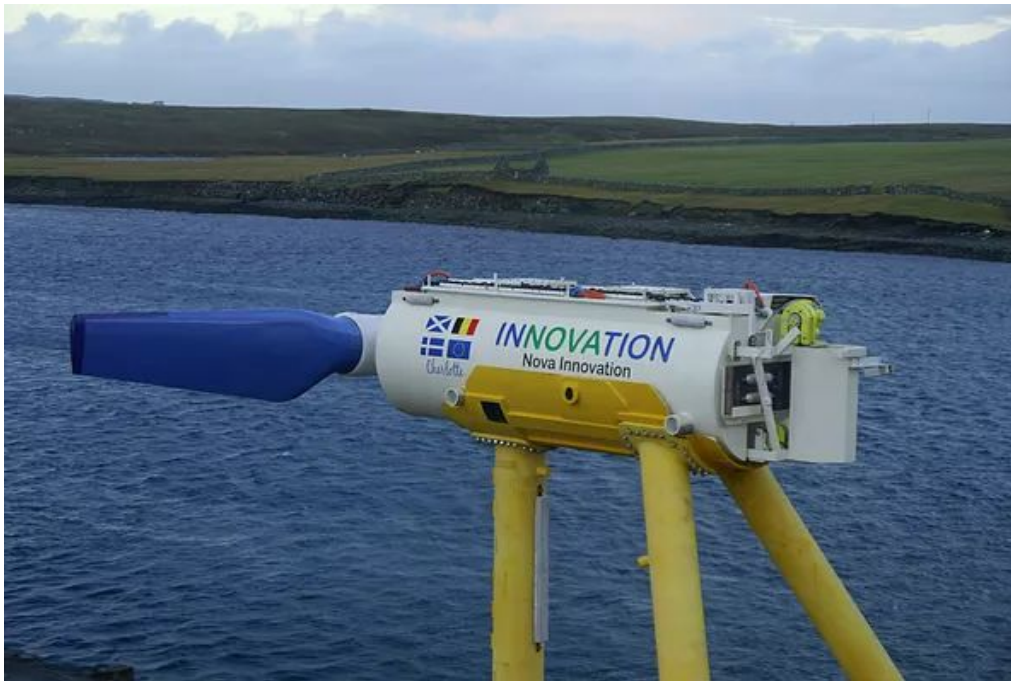
Figure 10: Nova M100 Horizontal Axis Tidal-Stream Turbine 12
