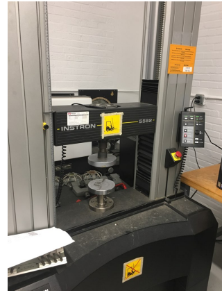
Figure 1: Instron model 5582 equipped with a 100kN load cell
