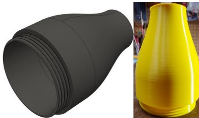
Figure 6.12: Nozzle V1 40 mm Outlet Diameter CAD Model and Prototype
