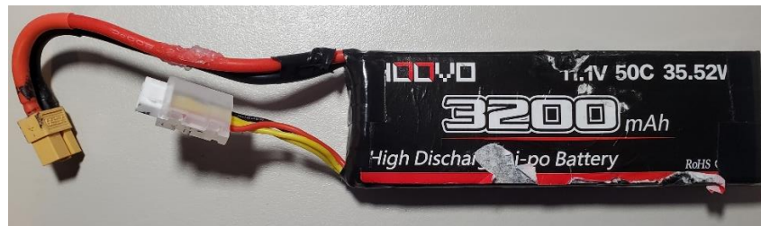
Figure 6.1: HOOVO 3S 11.1V 3200mAh 50C LiPo Battery
