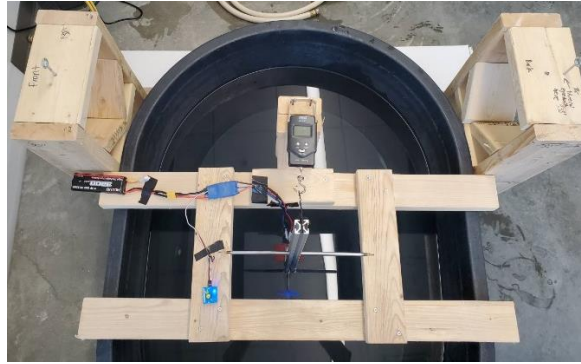
Figure 5.18: Testing Apparatus Assembled for Brushless Motor Testing
