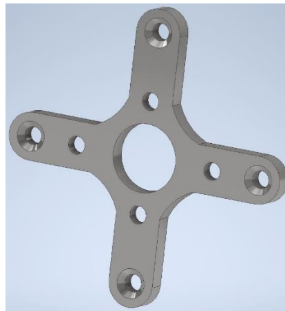
Figure 5.13: DYS 3548-5 Mounting Bracket
