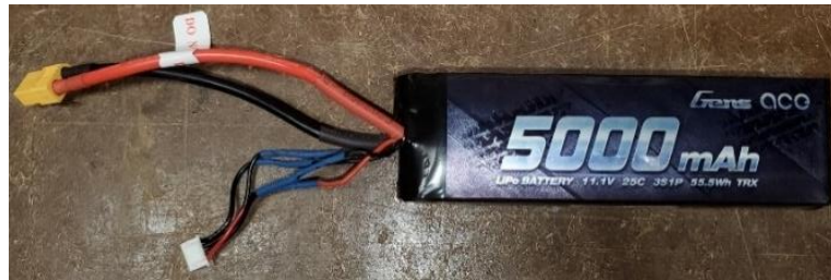
Figure 5.8: Gens Ace 5000mAh 11.1V 3S 25C LiPo Battery
